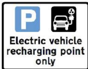
Figure 4: TSRGD compliant signage for EV charging bays (suitable on public highway and private roads)
